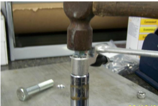
Using the hex headed bolt supplied simply tap the assembly down until you feel the resistance of the guide bearing setting on the socket face.
