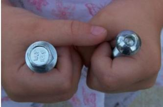
Use some removable thread locker and “snug” the bolt tight, yes I said “snug”. The purpose is to set the preload on the bearings and spacers. Once you feel resistance to the bolt turning, give it about an eighth of a turn more. If you are anal about such things, that should be 8 to 10 ft lbs.
