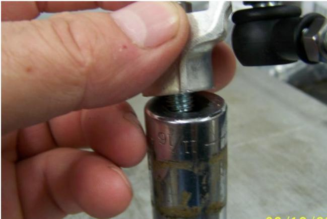
Notice this time we have the socket inverted and are driving into the 3/8 drive square hole.
