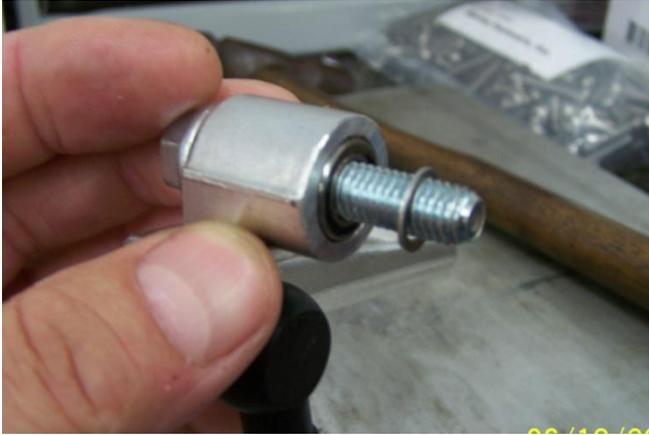
When you have the units seated, do not forget to install the thin stainless washer between the last bearing and the bracket it bolts to.
