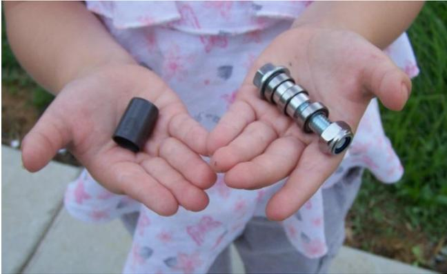
Factory OEM sleeve on the left, replacement parts on the right.
