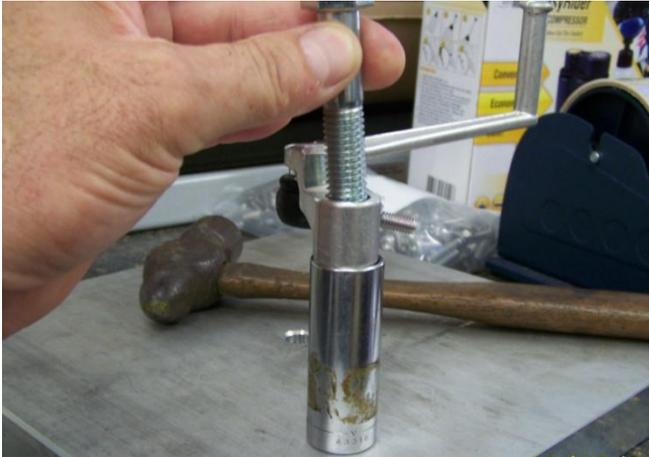
Support the bushing over the 5/8" socket opening and set the 1/2" bolt on top. You may want to "screw" the bolt into the bushing. Once in position, simply drive the bushing out.
