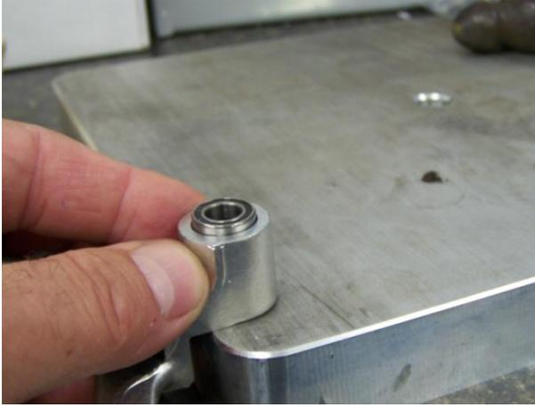
You can use the head of the ½" bolt to tap the bearing into position. A little tapping with a hammer on said bolt may be in order.
